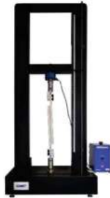
eXpert 2611 - 10kN Dual Column UTM Table top machine equipped with tensile composite shear fixture.
