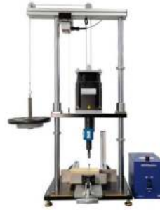
eXpert 8600 - 25Nm Vertical System Configured with rotary torque transducer and dead weight pulley system for recording torque while driving lag screws into wood.
