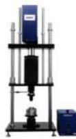
eXpert 8600 - ASTM F543 System Configured to test metallic medical bone screws according to ASTM F543 with the required fixturing for methods outlined in Annexes A1-A4. Force Capacity: 2.2 kN (500 lbf) Torque Capacity: 20 Nm (180 lbf-in)
