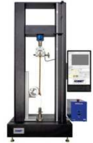
eXpert 2613 - 50kN Dual Column UTM Table top machine equipped with floating roller peel fixture and frame mounted touch panel computer.
