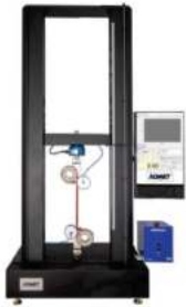
eXpert 2610 - 5kN Dual Column UTM Table top machine equipped with pneumatic rope grips and frame mounted touch panel computer.
