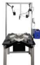
eXpert 8000 - Fatigue Planar Biaxial Force Capacity: 1 kN (225 lbf) Capable of force, displacement, strain control (using DIC system) in addition to sine, square, triangular cyclic waveforms, and independent or synchronized control of X & Y actuators
