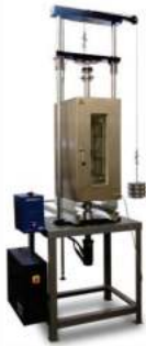
eXpert 8600 - 50Nm Vertical System Configured with -70^{\circ}\text{C} to 280^{\circ}\text{C} Environmental chamber and dead weight pulley system.
