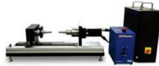
eXpert 8900 - 5Nm Fatigue System Configured with reaction torque transducer on sliding tail stock. System applies sinewave cyclic torque amplitude profiles up to 5Hz on UV sensitive polymer.
