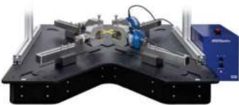
eXpert 8000 - Static Planar Biaxial Force Capacity: 5 kN (1,125 lbf) Capable of force, displacement, strain control (using DIC system) in addition to sine, square, triangular cyclic waveforms, and independent or synchronized control of X & Y actuators
