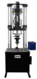
eXpert 8900 - Axial-Torsion Machine for Orthopedic Device Testing Engineered to perform both ASTM F2077 and F1717 on one system. Force Capacity: 17.5 kN (3,934 lbf) Torque Capacity: 80 Nm (708 lbf-in) Dynamic Capability: Up to 10 Hz Max Rotational Speed: 900 rpm
