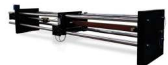
900kN Horizontal Pipe Tensile Tester This large custom servohydraulic system is engineered for customers who need to test entire pipe sections and their fusion welds. The system features a dual stage hydraulic power unit to allow faster speeds when jogging the actuator under no load conditions.
