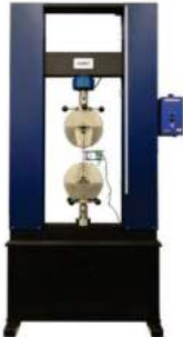
eXpert 2653 - 50kN Dual Column UTM Floor standing machine equipped with moving body wedge grips and extensometer.
