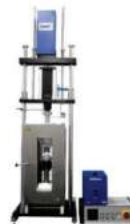
eXpert 8600 - Solid Ice Specimen Testing Designed to replicate artice conditions. Force Capacity: 5 kN (1,125 lbf) Torque Capacity: 50 Nm (445 lbf-in) Axial Speed: 0.0000254 - 9.14 in/min Rotational Speed: 0.0000003 - 0.01 RPM Features: Environmental Chamber
