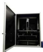
Solar Panel Bend Testing System The system includes a specialized bend fixture for solar cells, a camera to capture solar cell crack propagation, and the voltage drop is recorded by the controller to indicate cell damage. Axial Capacity: 5 kN (1,125 lbf) Features: Custom Blackout Safety Shield
